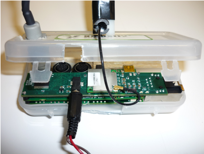
Figure 2.7: The gumstix in the box that is used to mount it on the hovercraft.
