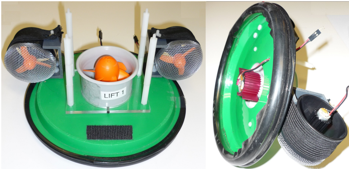
Figure 2.1: The hovercraft chassis.
