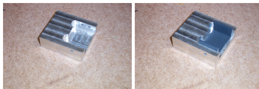
Figure 4: U-Channel Drill Fixture
