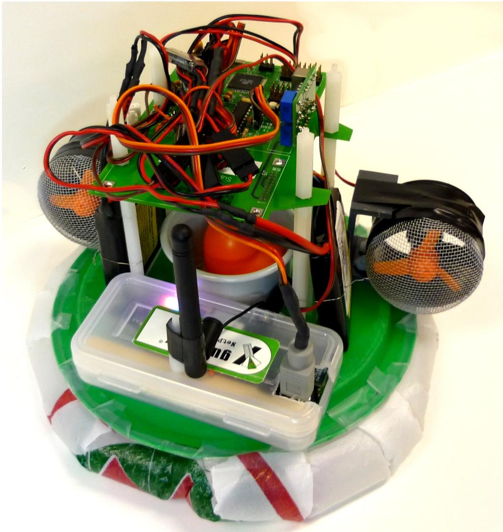
Figure 2.8: The assembled hovercraft (without the vision system hat).
