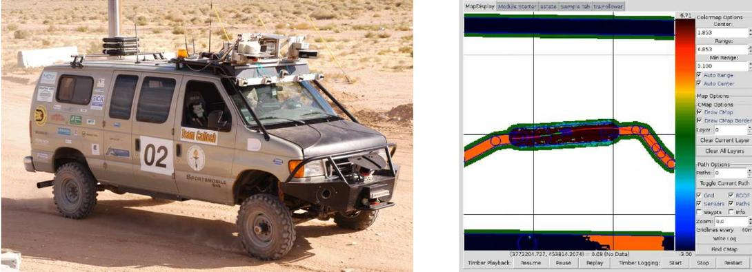
Figure 6: Caltech’s autonomous vehicle, Alice. The left figure shows the vehicle as configured for the 2005 DARPA Grand Challenge. The right figure shows the graphical user interface. The colors represent allowable speeds and the magenta line is the currently planned path.
