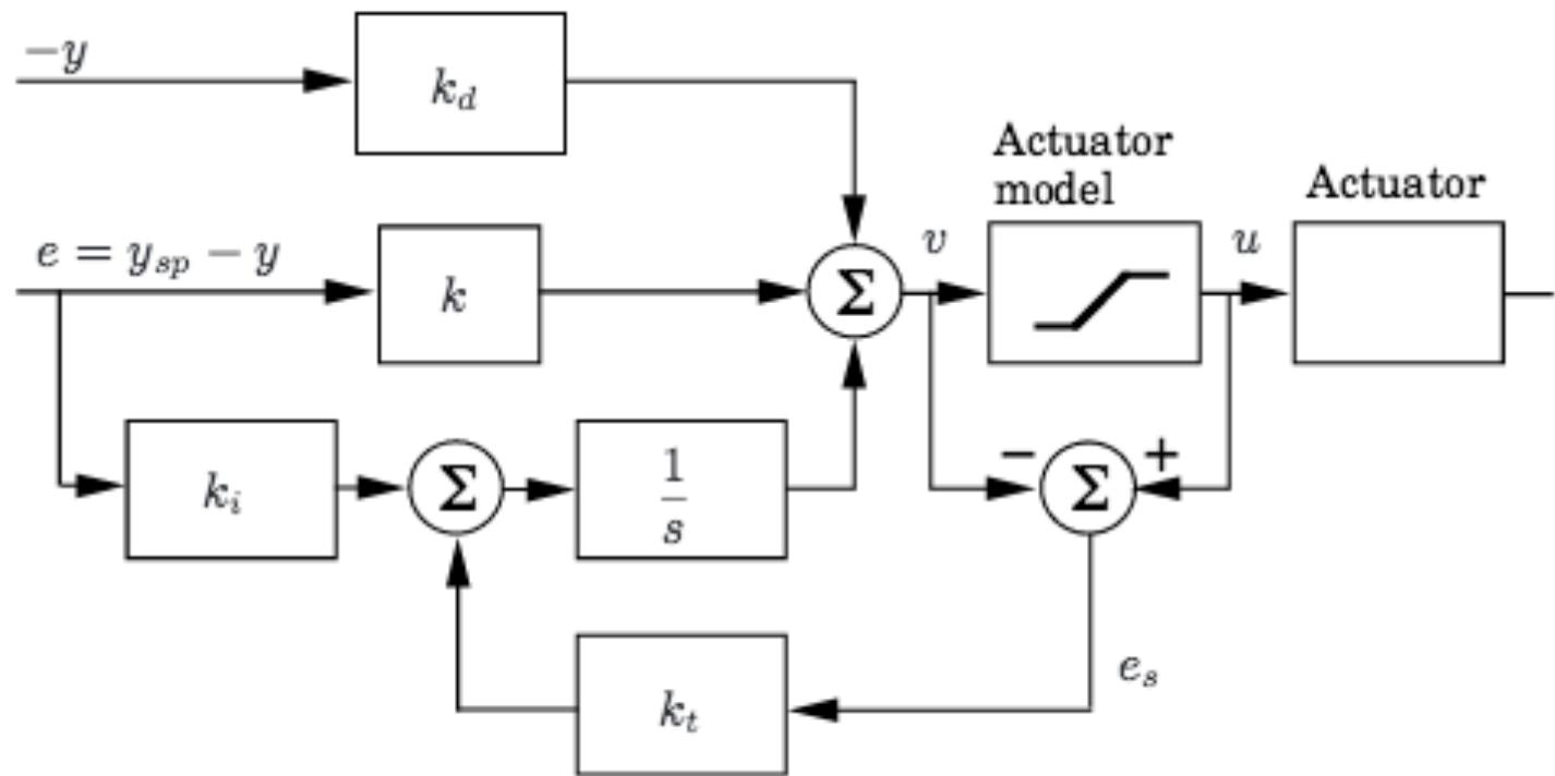
Figure 10.8: PID controller with anti-windup.
