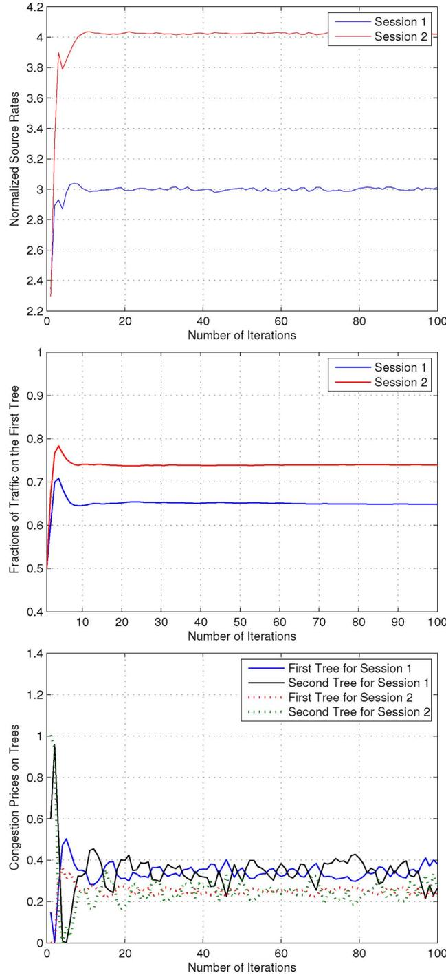
Fig. 4. Evolution of source rates (upper panel), the evolution of traffic split vectors (middle panel), and the evolution of congestion prices over different multicast trees (lower panel) versus the number of iterations of the tree adaptation algorithm with stepsize  $\delta t \kappa_m = 0.01$  for the example network with given coding subgraphs.
