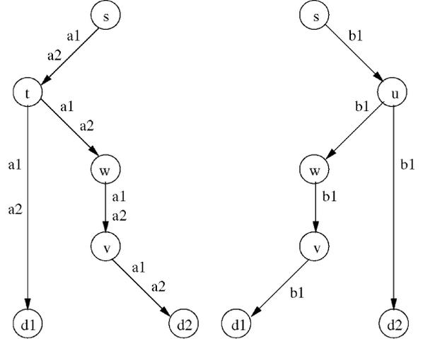
Fig. 2. Multicast trees for the example shown in Fig. 1. Coding is done on the shared link  $(w, v)$ , which, as part of the left tree, has one downstream destination  $d_2$ , and, as part of the right tree, has one downstream destination  $d_1$ . The left tree can support up to two units of information flow and the right tree can independently support up to one unit of information flow, since coding on link  $(w, v)$  allows the two trees to share capacity.
