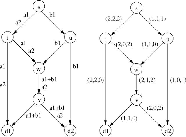
Fig. 1. Example network coding subgraph with one source  $s$  and two destinations  $d_1$  and  $d_2$  (left graph), where links  $(s, u)$ ,  $(u, w)$  and  $(u, d_2)$  are assumed to have one unit of capacity, and all other links have two units of capacity; and the corresponding flow variables (right graph), where each link  $(i, j)$  is marked by the triple  $(g_{i,j}, g_{i,j}^{d_1}, g_{i,j}^{d_2})$ .
