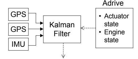
Vehicle position, orientation, velocities, accelerations
